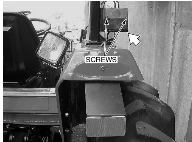
Figure 75 - Tail Light and Flasher Warning Lights
