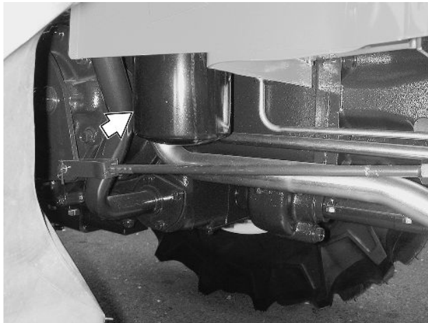
Figure 58 - Hydraulic Oil Filter
