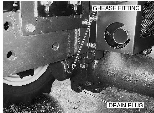
Figure 82 - Front Axle Differential Drain Plug and Grease Fitting
