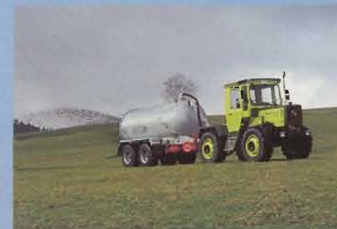
The four-wheel braking system is the only answer on steep slopes and wet grass.
