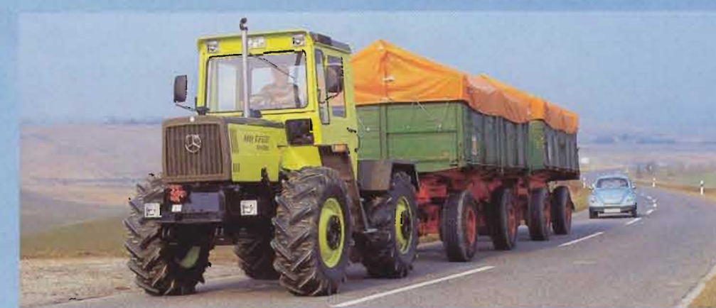
Because of its four-wheel braking system the MB-trac can be stopped quickly and with low pedal pressures, even in critical situations.
