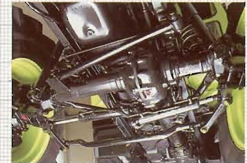
The strong front axle – being the same design as the rear axle – offers high load capacity for heavy front implements.
