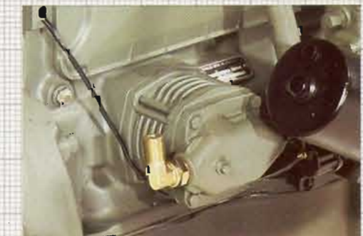
The maintenance-free and reliable engine-mounted compressor provides auxiliary power for the braking system.
