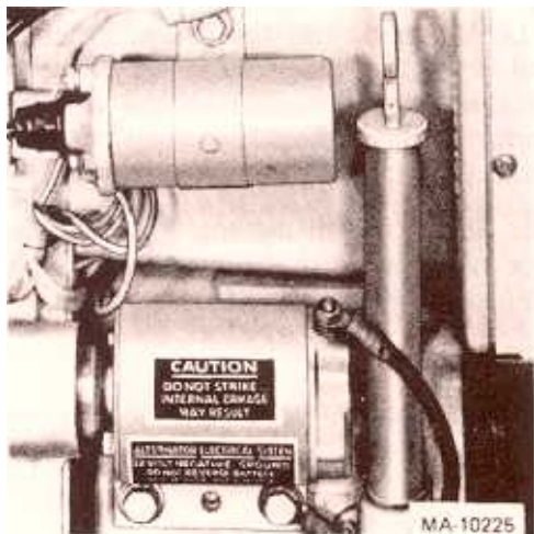
1. Oil filler cap and oil level gauge - All models except the Cub Cadet 800 Tractor
