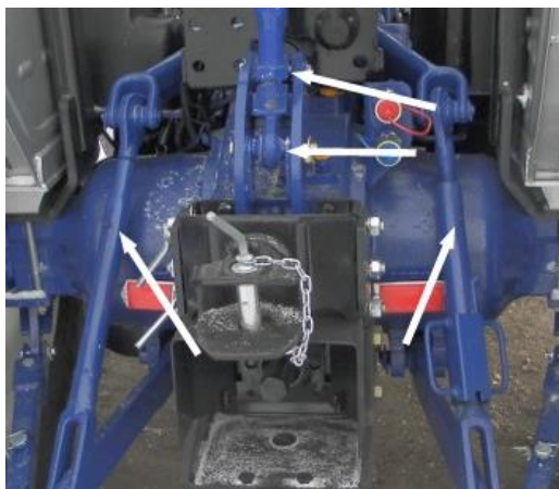
Fig. 5.10 Three-point linkage greasing fittings.
