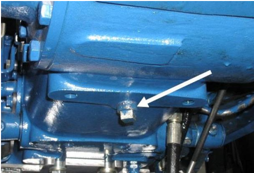
Fig. 5.9.1. Rear axle oil drain plug.
