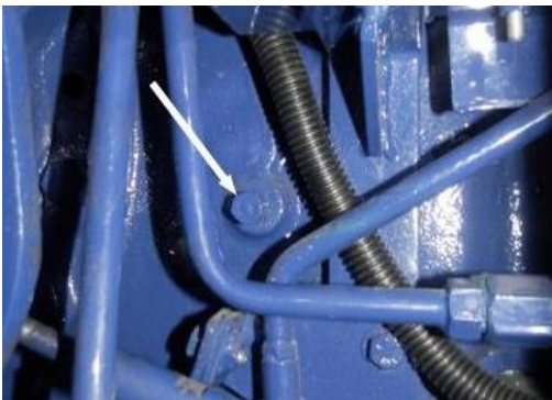
Fig. 5.9.5. Rear axle oil level control plug.
