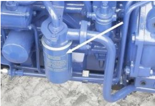
Fig. 5.9.3. Hydraulic oil filter.
