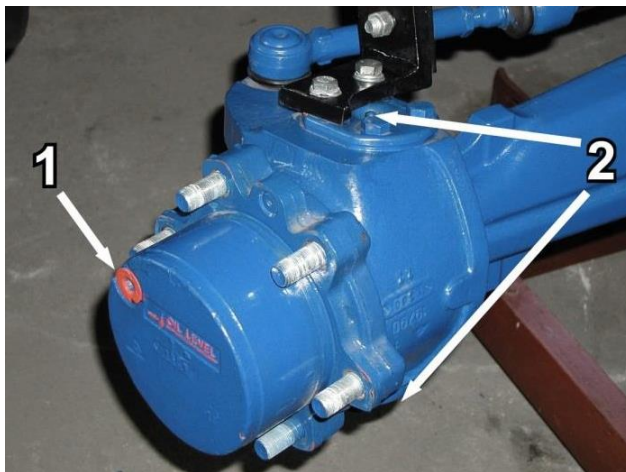
Fig. 5.6.2. Epicyclic reduction unit of front drive axle. 1 - Filler/level/drain plug. 2 - King pin grease points (2 pcs. on each side of tractor – at the top and at the bottom).
