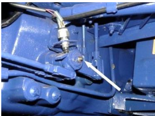
Fig. 5.12.1 Brake system actuation mechanism grease fitting.
