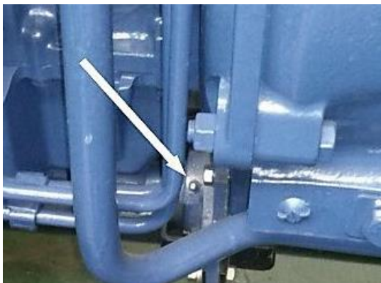
Fig. 5.7.9. Propeller shaft of front drive axle – grease point.
