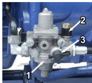
Fig. 5.13.4. Air Pressure regulating valve. 1-Air regulating valve. 2-Safety valve. 3-Tyre inflating valve
