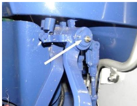
Fig. 5.12.2 Brake pivot grease fitting.
