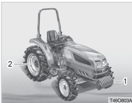
(1) Front End Weights (2) Rear Wheel Weights
