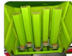
Long length straw walkers for complete separation of grains and straw.
