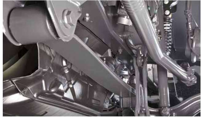
Front spring, 3.4 t, parabolic (Q1C)
