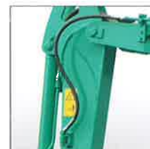
Auxiliary Hydraulic Piping
