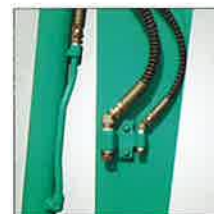
Auxiliary Hydraulic Piping & 2nd Auxiliary Piping
