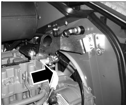
Fig. 127: Cleaning the oil cooler
