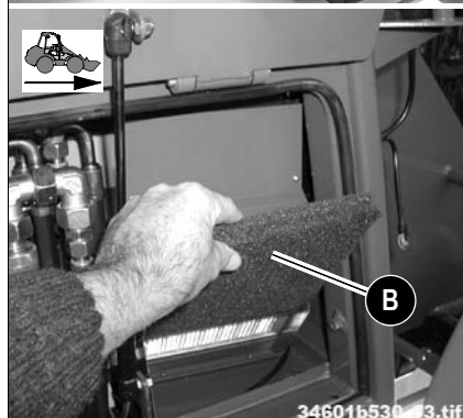
Fig. 147: Replacing the dust filter of the heating system
