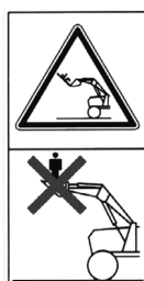
Fig. 21: Prohibiting sign: transport of persons
