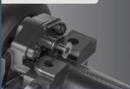
Clutch wear indicator
