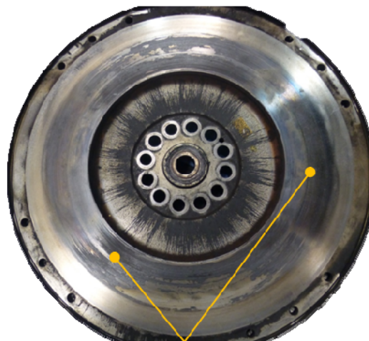
Grease and Disc Material Transfer on Flywheel Face
