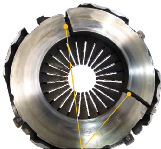
Pressure Plate Fractured
