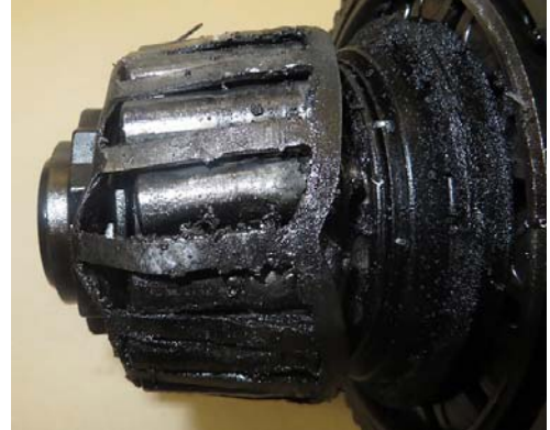
Mainshaft Pilot Bearing Damaged
