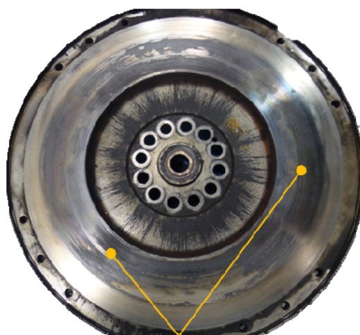
Grease and Disc Material Transfer on Flywheel Face
