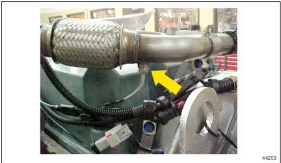
Figure 2-13 EGR Temperature Sensor
