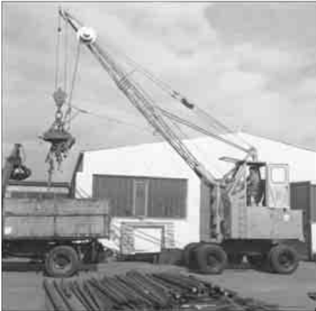
1962: Rope-driven S833 with elevated operator cab
