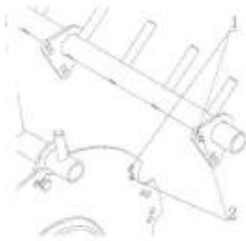
Figure 8 Adjustment of the concave plate gap
