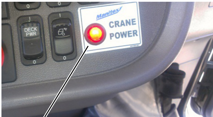
Crane Power Switch 2-Pos ON/OFF
