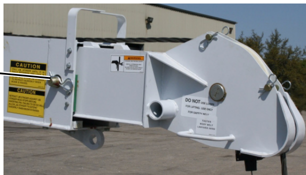
Figure 2-27 Pin 6 installed to lock stinger in place
