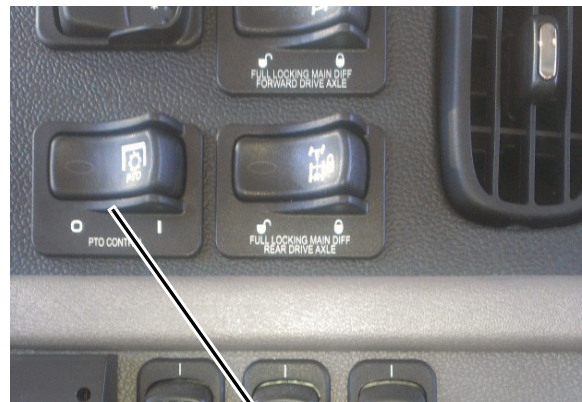
PTO Switch 2-Pos ON/OFF
