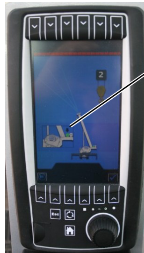
Arrow above Main or Auxiliary winch indicates current selection.
