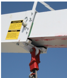
Load line attached to lug at tip end of jib base
