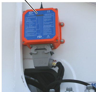
2 - Indicator lights Receiver located on the turret.
