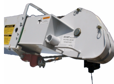
Stinger retracted using jib load line
