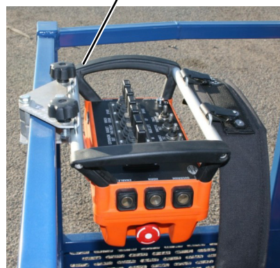
Controller secured in place in basket for aerial operations.
