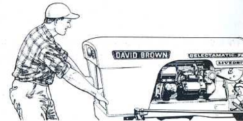
FIGURE 3/1. LIFTING THE BONNET FROM THE FRONT EXTENSION.
