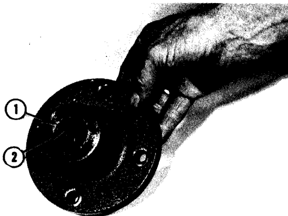
FIG. 10.7--BEARING AND SEAL INSTALLED
