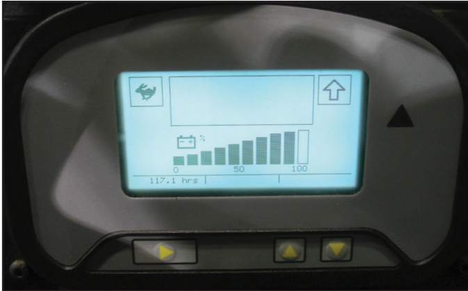
Dash Display with Full Diagnostics Battery Discharge Indicator and Hour Meter
