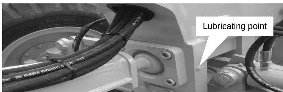
Fig.8 Lubricating point of ball socket
