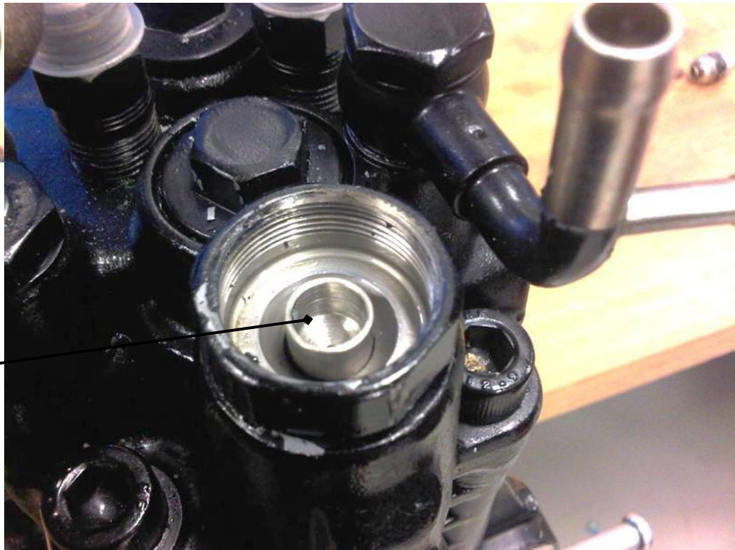
Timer cap installed
