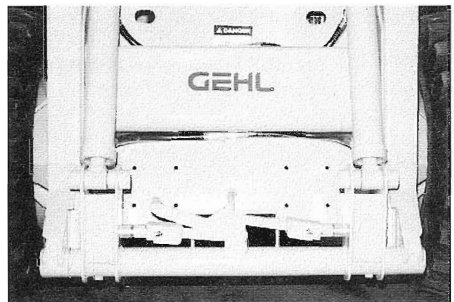
Fig. 11: Quick-Tach Lever in "Release" Position all the way to the Right (Attachment Removed for Clarity)
