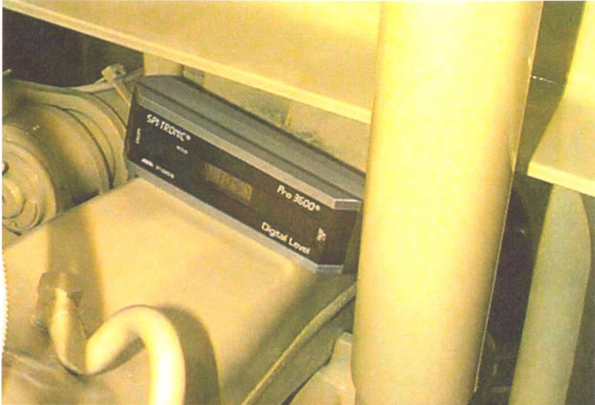
Figure 10 Illustration of Using an Inclinometer to Determine Rear Rear Axle Angle
