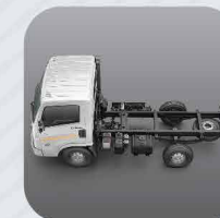
CED coated rust resistant, sturdier & rugged BSK46 chassis
