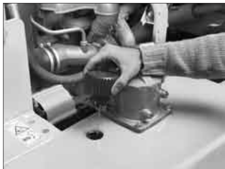
Fig. 68 Reducing residual pressure
