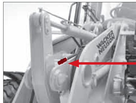
Fig. 45 Depressurized return line
