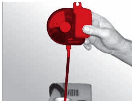
Fig. 87 Checking the anti-freeze mix
