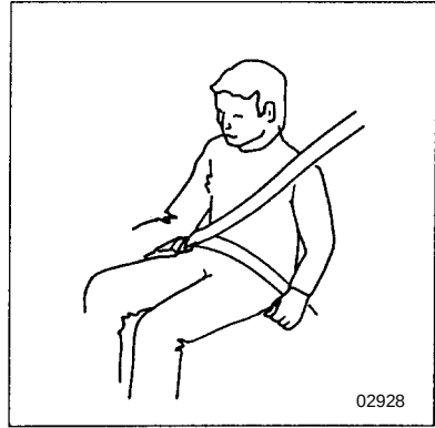
Improperly worn belt
