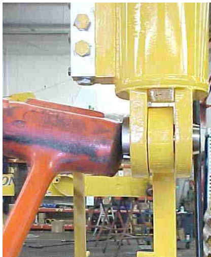
DRIVE PIN THROUGH AND SECURE WITH CAPSCREW AND NUT. USE LOCKTIGHT ON CAPSCREW BEFORE INSERTING AND TORQUE TO PROPER SPECS.
