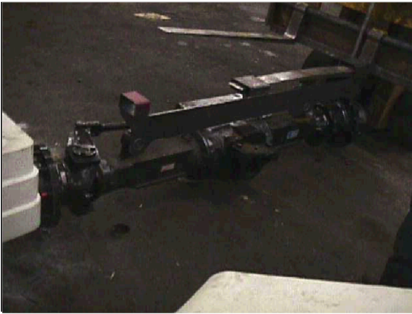
MOVING REAR AXLE INTO PLACE
