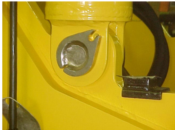
LIFT CYLINDER BASE PIN
