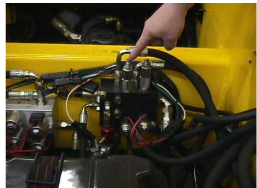
Brake manifold/Pilot adjust screw
