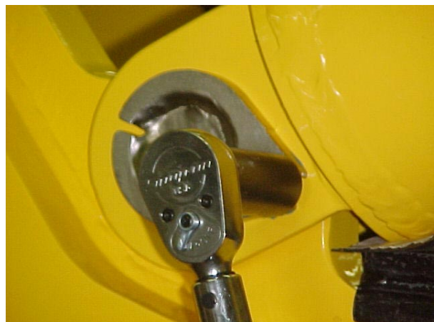
TORQUE CAPSCREW TO PROPER SPECIFICATION.
