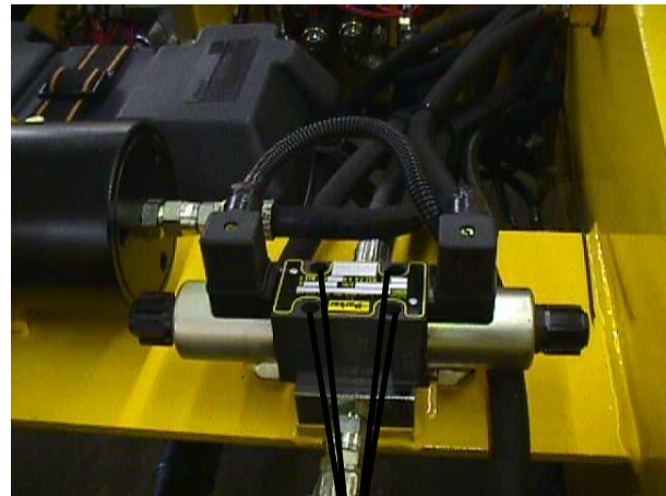
VALVE BODY TO VALVE BLOCK SCREWS
