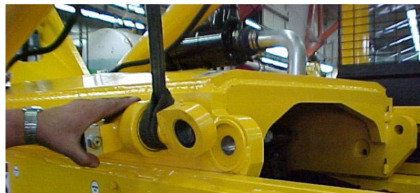
RE-LOCATION OF LIFTING STRAP AND LINING UP OF THE FRONT MOUNT.
