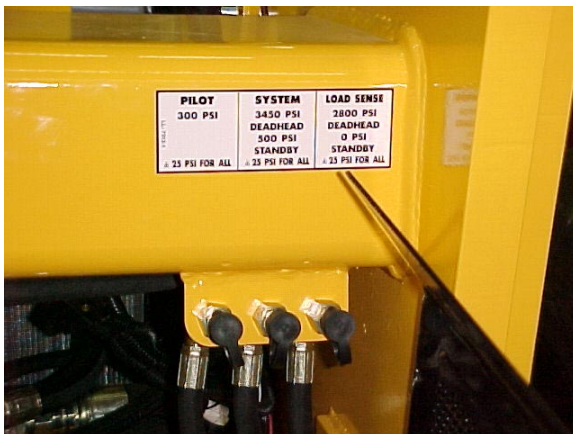
Pressure Checks, Valve in Back
