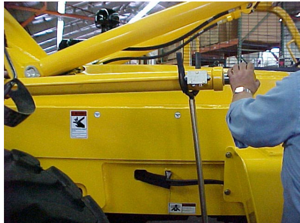
PLACING CYLINDER ON STAND.
