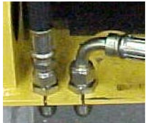
FIXED MACHINE BULKHEAD FITTINGS
