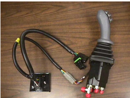
Fork Tilt and Auxiliary Function Joystick with Digital PWM Module
