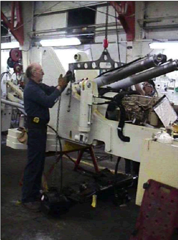
ATTACHING SLING AND CHAINS LIFTING AXLE
