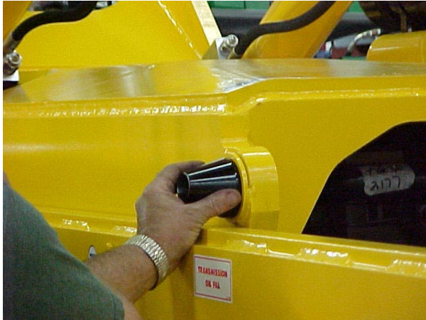
POSITIONING THE FRONT MOUNTING CONE.
