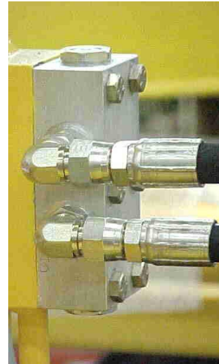
CONNECT HYDRAULIC LINES TO CYLINDER
