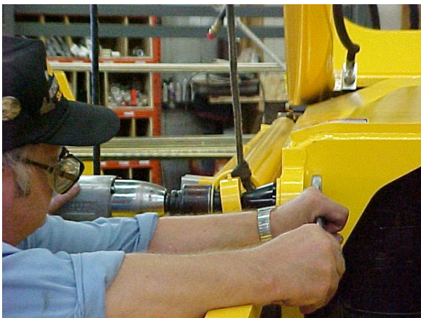
TIGHTENING OF FRONT BOLT AND NUT.
