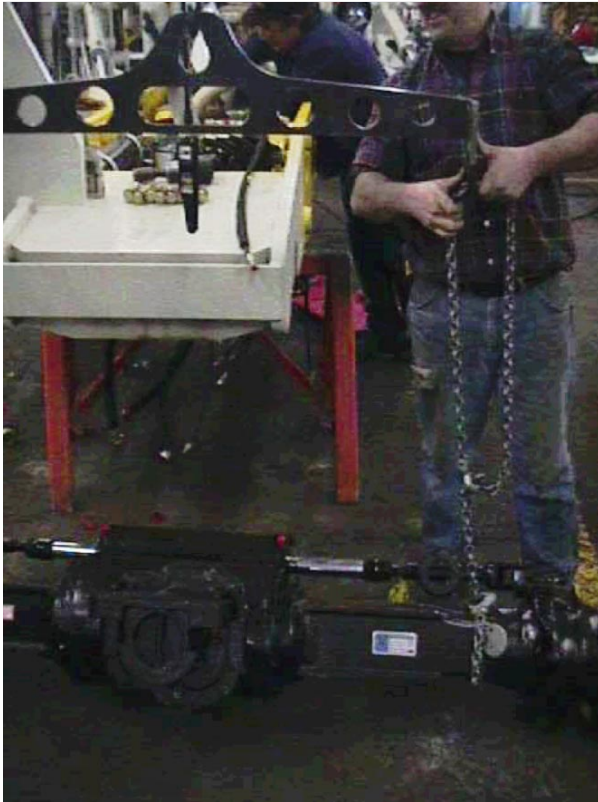
ATTACHING SLING AND CHAINS LIFTING AXLE
