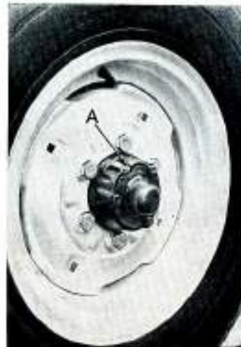
FIGURE 3/13. FRONT HUB A. Front hub greaser (filling)
