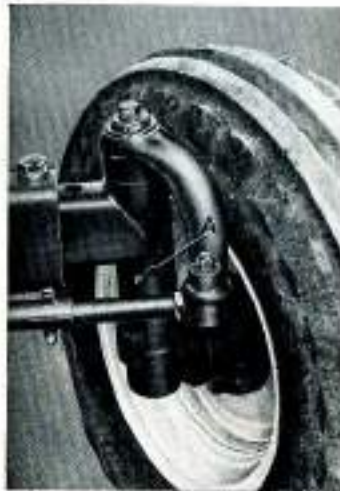
FIGURE 3/12. FRONT AXLE A. King pin lubrication point
