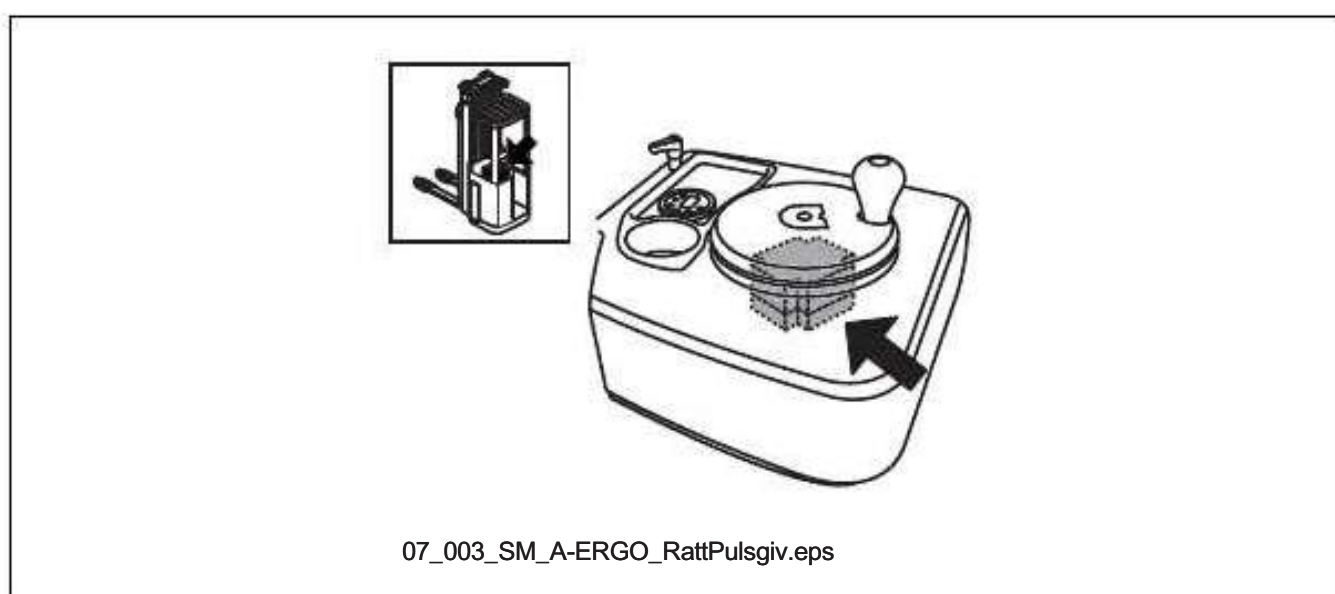
Figure 7.2 Position of step motor sensor
