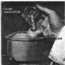
Fig. 30. Checking Pump Reservoir Oil Level
