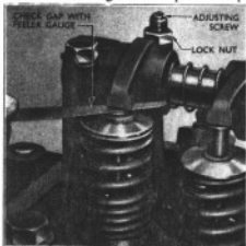
Fig. 12. Valve Tappet Adjustment
