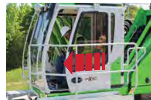
maXCab's sliding door and guarded permanent catwalk provides the safest entry and exit in the industry.
