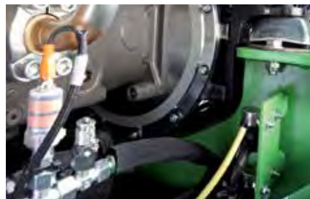
Low-vibration engine mounting reduces wear on components and lowers sound levels.
