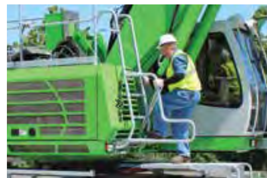
Permanent 3-point contact for access to upper deck with full railings and anti-slip walking surfaces to protect service crews during inspections and repairs.
