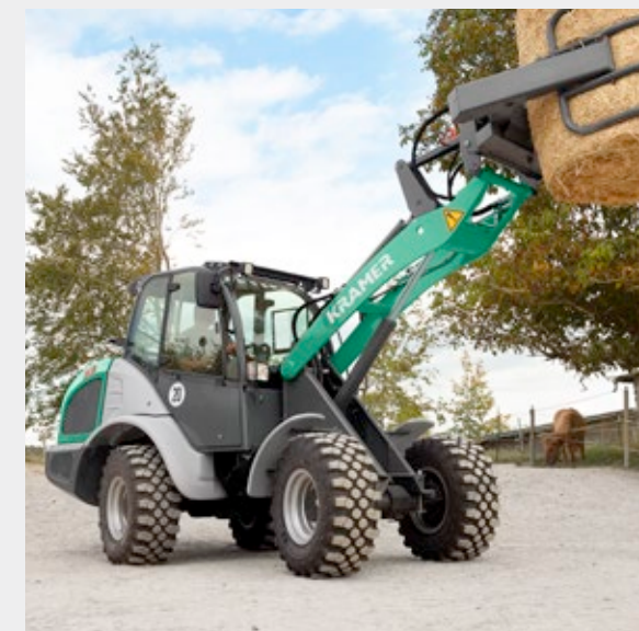
Crab steering for precise positioning
