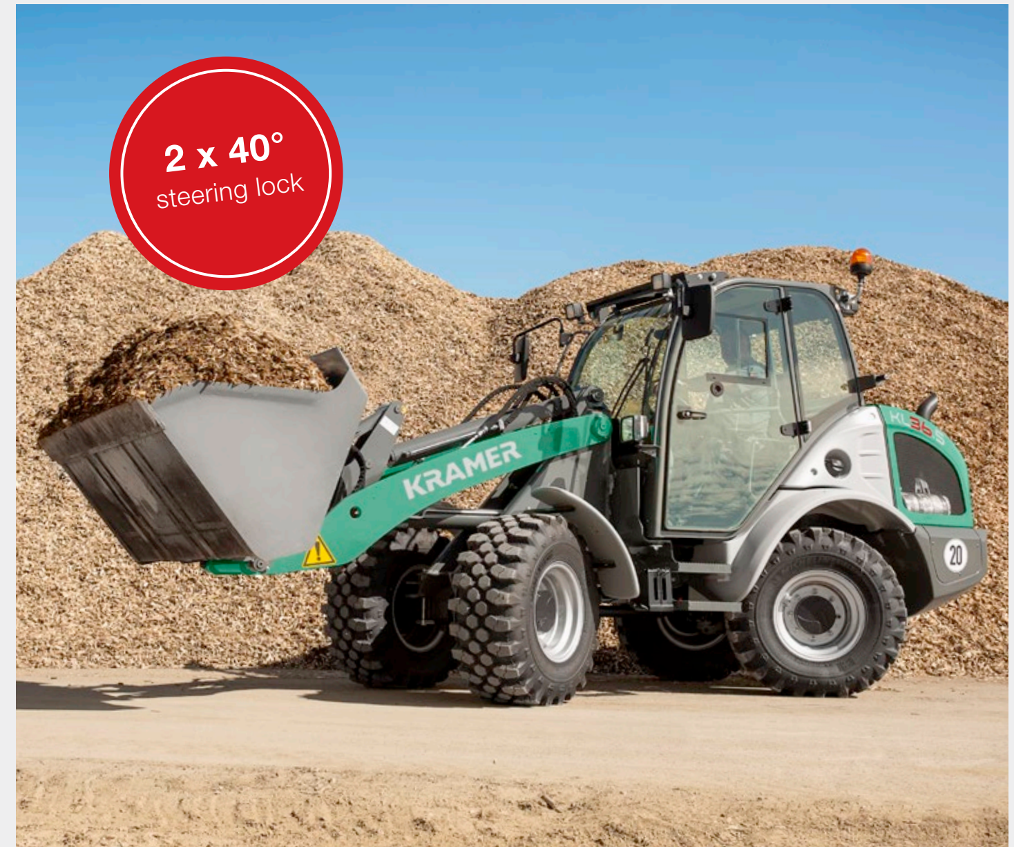
All-wheel steering is particularly manoeuvrable in tight spaces
