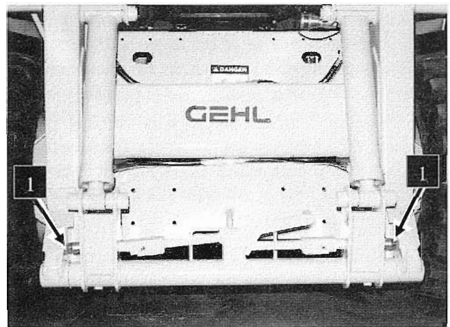
Fig. 10: Quick Tach Lever in "Engaged" Position all the way to the Left (Attachment Removed for Clarity)
