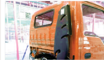
R.H.S. Vertical Air Cleaner for Better Air Filtrations
