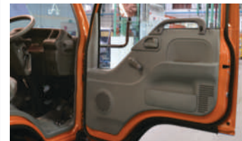
Wide Door Aperture (~90° Angle Approx) & Antiskid Footstep for Easy Inlet/Outlet
