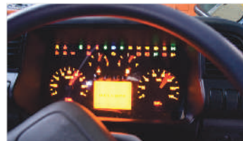
CAN Based Meter Cluster with Multi-Info Display
