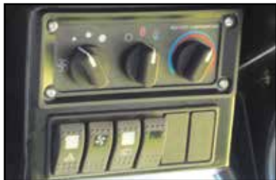
Cab heater with defroster and fan. Optional air conditioning unit available.
