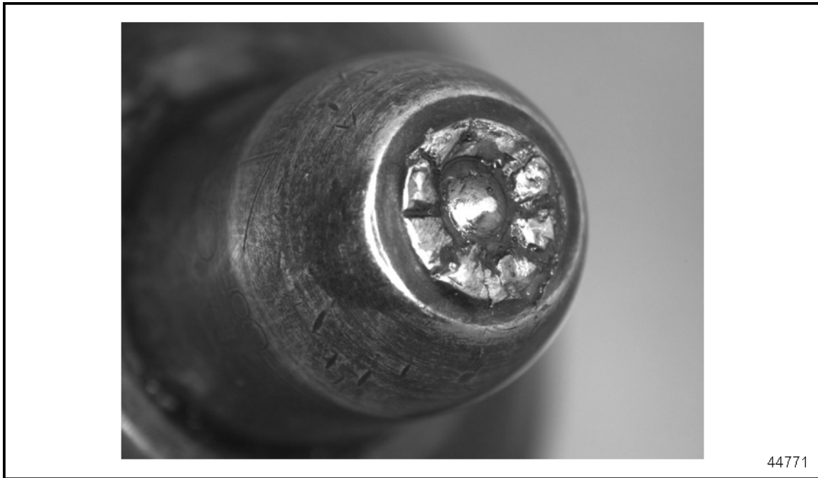
Figure 6-8 Failed or Blown Spray Tip Failure
