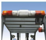
High Mounted Rear Combination and Beacon Lights.
