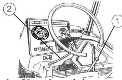
Shifting the GB with single-lever control and a multiplier (accelerator);
