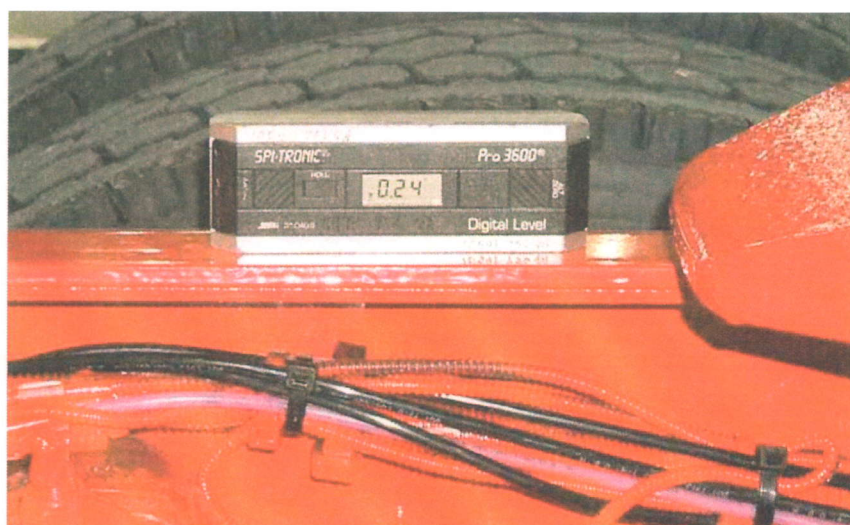
Figure 8 Illustration of Inclinometer on the Left-Hand Frame Rail
