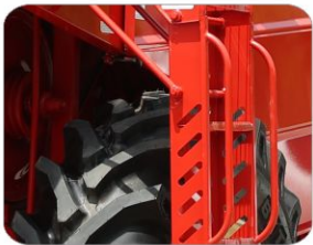
Ladder cover with sheet for safety purpose
