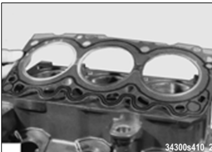
Fig. 118: Placing the cylinder-head gasket
