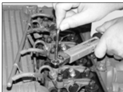
Fig. 91: Setting valve clearance
