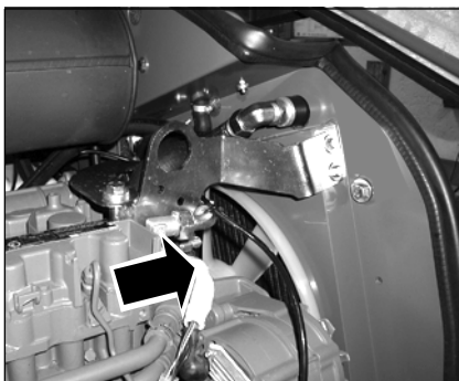
Fig. 57: Cleaning the oil cooler
