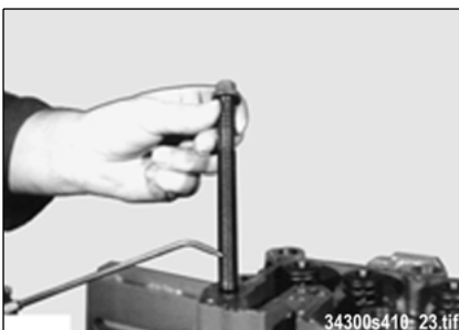
Fig. 119: Placing the cylinder-head gasket
