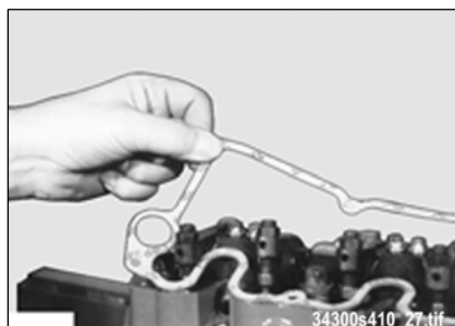
Fig. 123: Mounting the cylinder-head cover
