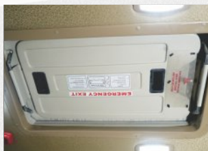
Two Emergency Exit Roof Hatches
