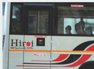
Emergency Exit Door
