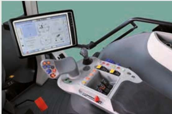
Cab with Premium version: the controls of the VT-Drive transmission are integrated into the armrest of the driver's seat.
