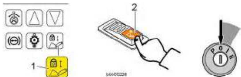
Working hydraulics lockout
