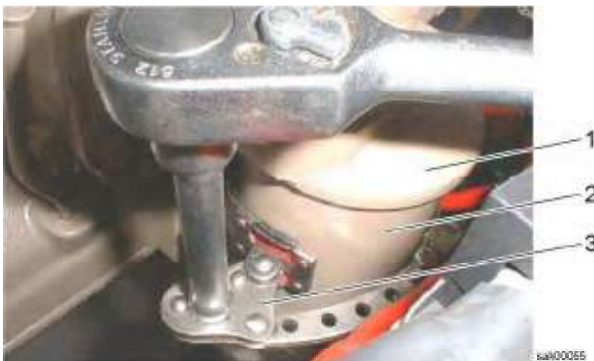
Unscrewing the oil filter
