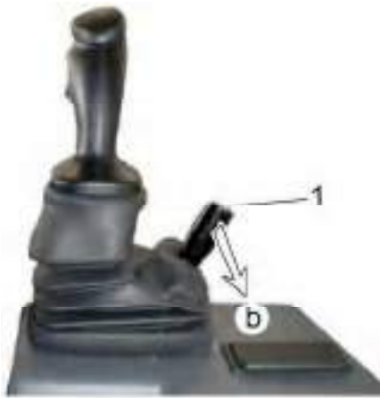
Unlocking the quick-change device
