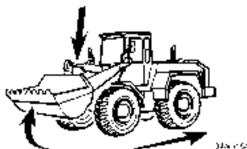
Lift arm position.
