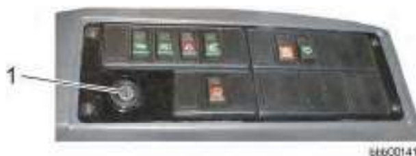
Ignition switch position
