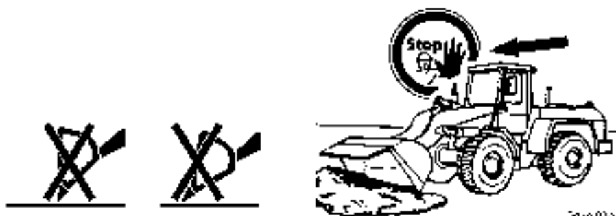
Impermissible bucket positions
