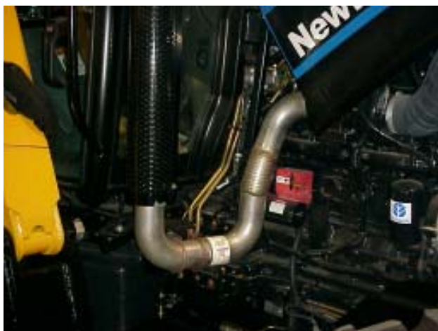
Figure 1: Replacement Exhaust Pipe (Elbow) & Bracket
