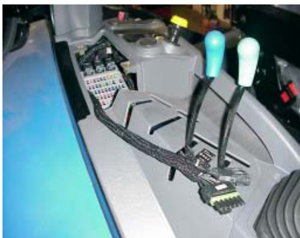
Figure 5: Electronic Module mounted & unseen behind cab panel
