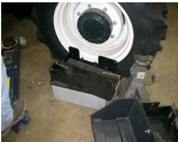
Figure 3: Battery Box Clearance
