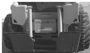
Figure 14 All-Tach™ Attaching Mechanism (Hitch)
