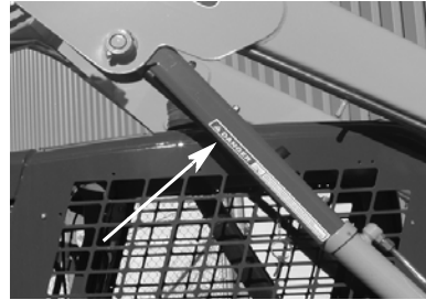
Figure 4 Lift Arm Support Device Engaged
