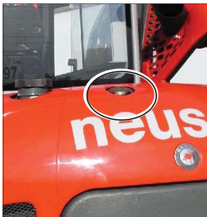
Fig. 40: Hydraulic oil filler inlet with strainer
