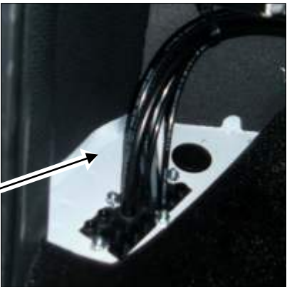
Cab pass through manifold located behind driver side dead pedal
