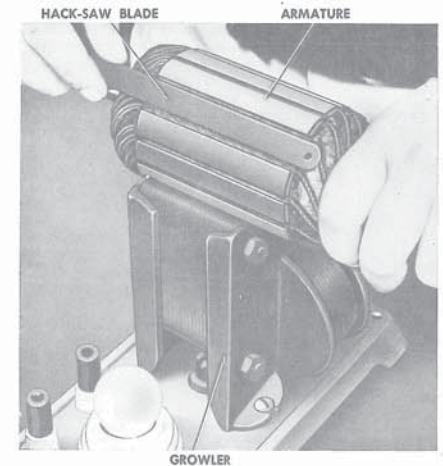
Fig. 38. Testing Armature in a Growler
