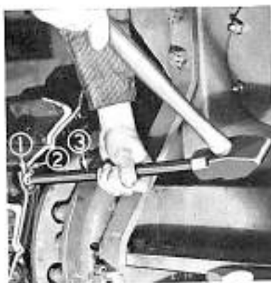
1. MASTER TRACK PIN 2. SLOT FOR LOCK PIN 3. DRIFT
