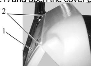
1 – cover of instrument board; 2 – screw.
